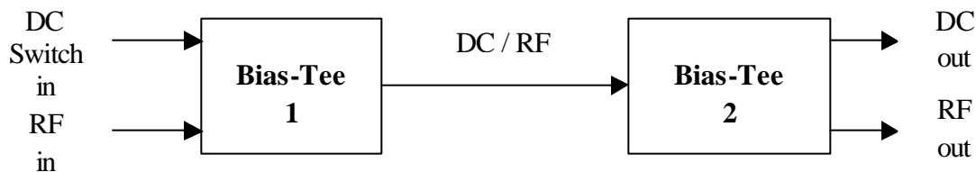
Figure 1: MFJ-4117 Bias-Tee Operation Diagram
